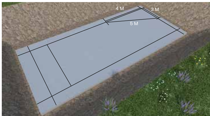
1 Draw the swimming pool with the inside measurements
